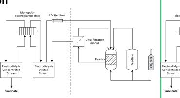
Figure 1: Schematic process flow of producing "green" succinic acid of an integrated membrane-bioreactor-electrodialysis system
