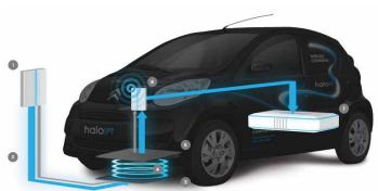
Image 1: The haloIPT wireless charging system. 1 – Power supply. 2 – Electrical wires. 3 – Transmitter pad. 4 – Wireless electricity transfer. 5 – Receiver pad. 6 – Data receiver. 7 – Battery <sup>7</sup>.
