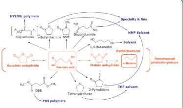
Figure 1: The diverse chemical synthesis opportunities offered by using succinic acid as a building block chemical
