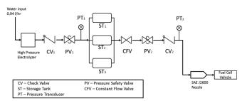
Figure 1: Major components of a residential hydrogen filling station. Redrawn from [1]
