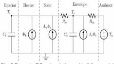
Fig. 2 Example RC-network thermal building model
