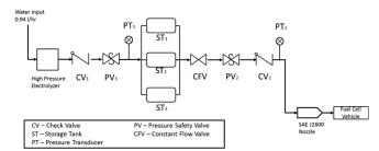
Figure 1: Major components of a residential hydrogen filling station. Redrawn from [1]
