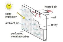
Figure 3 Example of an unglazed thermal solar wall
