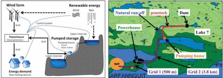
Schematic drawing of the supply system
