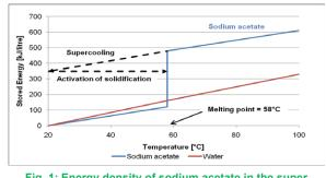
Fig. 1: Energy density of sodium acetate in the super cooling process compared to water.
