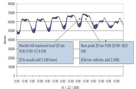
Example of coordinated (smart) charging in Nordic power system: The peak load moves to next hour (compared to case of no EVs). Load follows same pattern during time period making better use of Nordic power production capacity [1]
