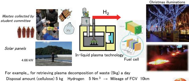
Jisposal amount (cellulose) 5 kg Hydrogen 5 Nm <sup>3</sup> → Mil + Carbon 1kg Solar cell system 5kW (Source) Nomura Shinfuku, 2013
